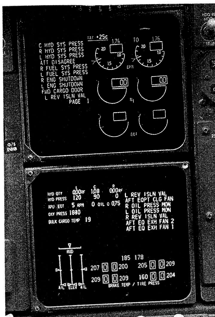
Figure 1.19 Boeing 757 EICAS display
