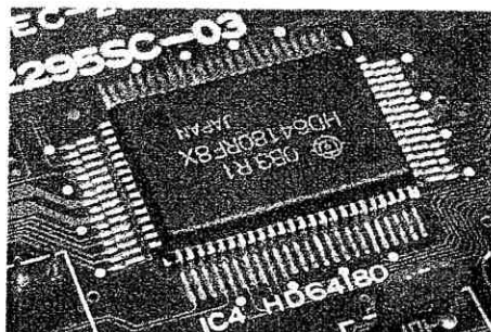
Figure 8.3 An 8-bit CMOS microprocessor supplied in an 80-pin plastic quad flat package (PQFP)
