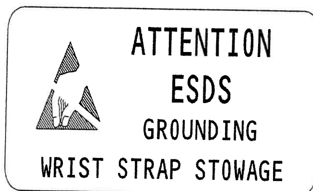
Figure 12.7 ESD wrist strap stowage notice
